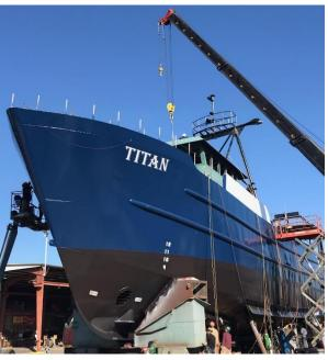
The 121' F/V TITAN was hauled out for conversion on January 12th 2018. The vessel was completely gutted of all equipment systems including; piping, wiring, mechanical, electrical, hull insulation, and all accommodations (walls, flooring, galley etc.). The pilothouse and all rigging (mast, booms and outriggers) were also removed.
