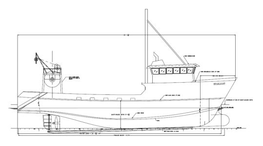
The **STARLIGHT** will be hauled out this month to begin cutting away the bow, pilothouse, and other areas of the hull. The new stainless steel pilothouse is constructed and ready, while the new bow module is currently under construction. Prefabrication of the new hull sponsons are now underway.
