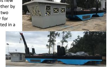
for work. The two hulls are independent but pinned together to work as one with a bolt-on elevated pilot house for larger inaccessible projects.
