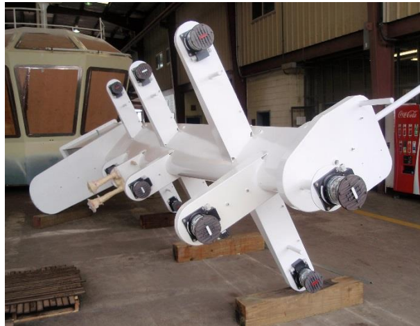
Aluminum mast in main shop for outfitting.
