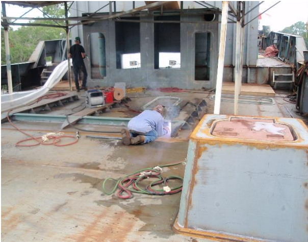
Mark and Huu on the aft deck completing the main winch foundation.
