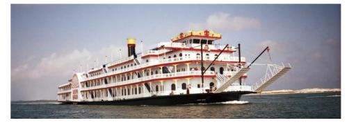
East St. Louis "CASINO QUEEN" The largest gambling vessel built at that time. 4,000 passenger, 850 slot machines, 7 bars, 3 elevators, triple screw and 4 thrusters.
