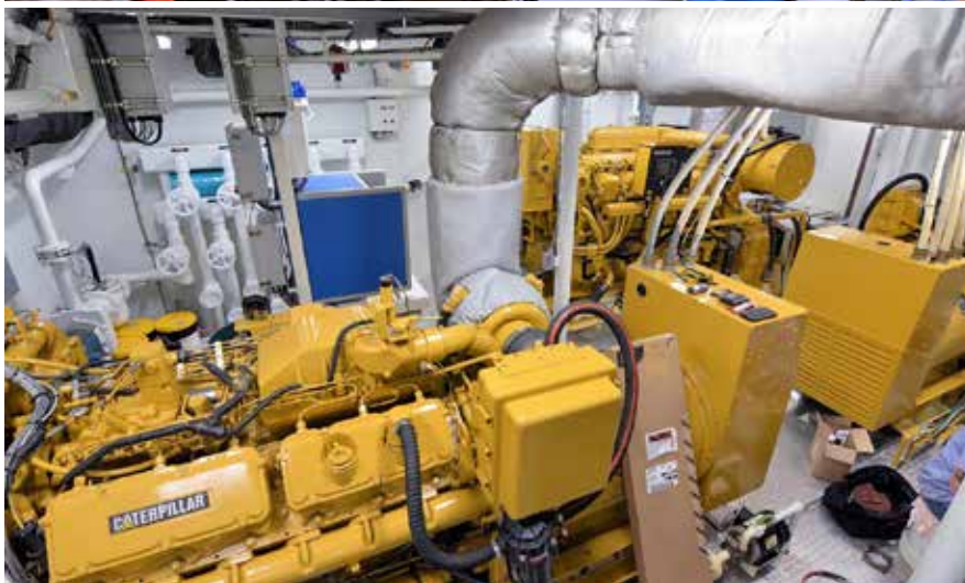
(TOP) The hydraulic room boasts the ten ABB electric motors. (ABOVE) The Caterpillar 3512 mains were rebuilt in place, and each provide 1,800 HP to ZF W7500 4.939:1 reduction gears turning 81-inch propellers inside new nozzles for a cruising speed with full tanks of 10.5 knots. Photos by Peter Marsh.
