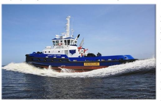
buoys on the Mississippi River and connecting waterway systems. The third delivery was the **Signet Polaris**. This 105', 6,800 horsepower "Z"-Drive Tug was the second (sister) tug for Signet Maritime. Both tugs were designed by the renowned Canadian firm of
