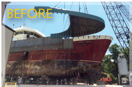
▲ The Western Venture's forward deck is being enclosed with bulwarks and a whaleback top deck is lowered in place.
