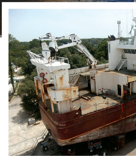
▲ The Western Venture before being lengthened 6 feet at the stern for working area around the net reels.
