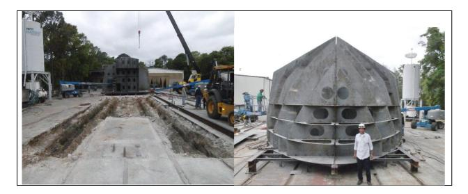
Modular work has begun on the construction of our latest project for the Moran Towing Co. This 6,000 horsepower ATB Tug is designed for handling ocean going barges in full ocean service in both pushing mode and towing astern. It is specifically built to be connected to a 450' barge, also under construction at another facility. This tug and barge interconnecting system forms an articulated tug/barge unit or ATB.
