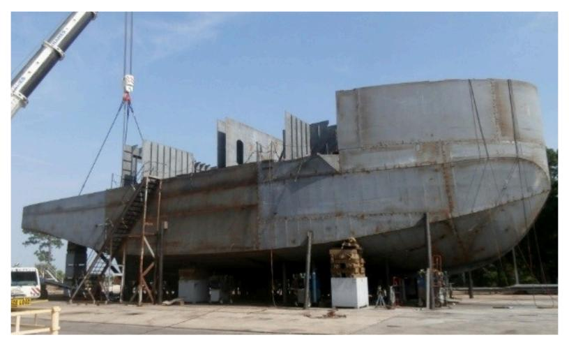
Patti Marine has completed the erection of the Moran 121' ATB hull modules with the stern installation this week. Deep South's 600 Ton Hydraulic Crane flipped and set the 207,000 lb. unit which completed the 3 month long hull erection process. Both main engines (6,000 horsepower EMD's) are already installed in the engine room. Our "Patti Built" crews have again proved their worth in speed and high quality workmanship!
