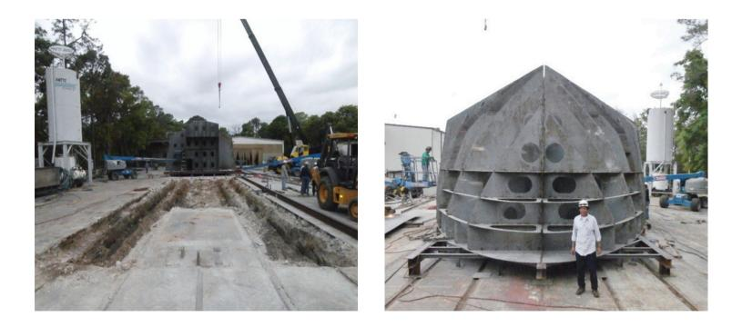
Modular work has begun on the construction of our latest project for the Moran Towing Co. This 6,000 horsepower ATB Tug is designed for handling ocean going barges in full ocean service in both pushing mode and towing astern. It is specifically built to be connected to a 450' barge, also under construction at another facility. This tug and barge interconnecting system forms an articulated tug/barge unit or ATB.
